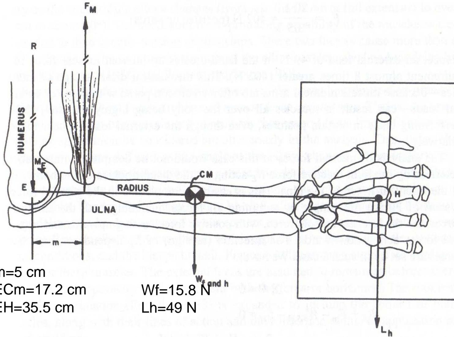
$$W_f \times E_{cm} + L_h \times E_H = F_m \times m = (15.8 \times 17.2 \text{ N cm} + 49 \times 35.5 \text{ N cm}) = 20.1 \text{ Nm}$$
