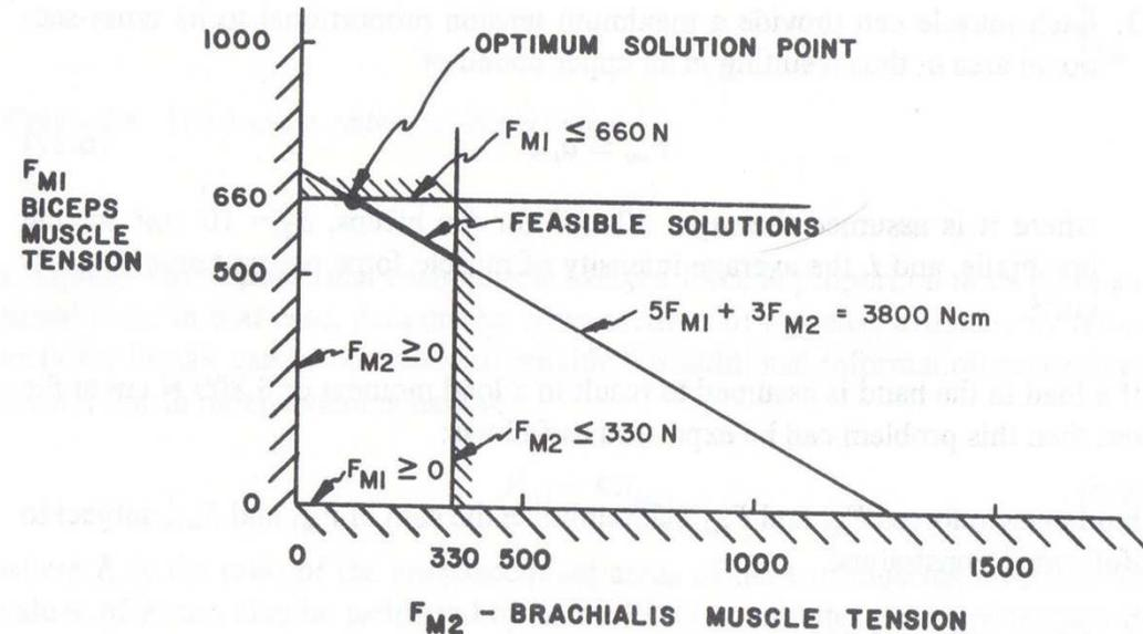
$$\begin{cases} 5F_{m1} + 3F_{m2} = 3800 \text{ Ncm} \\ F_{m1} \leq 660 \text{ N} \\ F_{m2} \leq 330 \text{ N} \end{cases}$$
