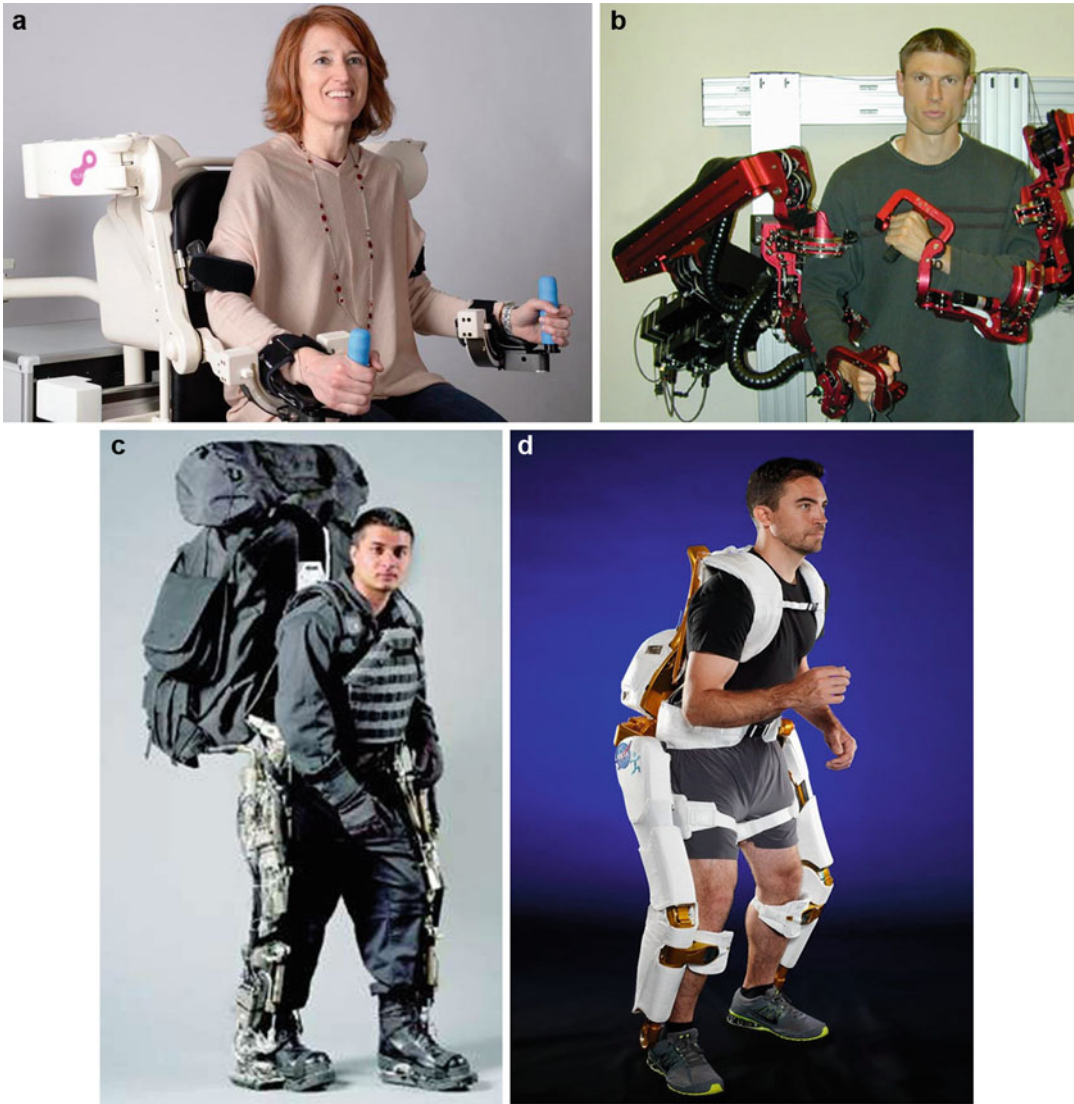
Wearable Robots, Fig. 2 Some examples of ULEs and LLEs. (a) The Alex exoskeleton (Pirondini et al. 2016). (b) CADEN-7 exoskeleton (Perry et al. 2007). (c) Hulk
